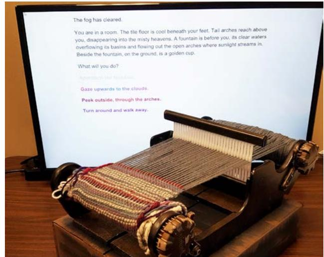
**Figure 1. The loom controller with the game displaying behind it. The electronics are hidden in the base.**
